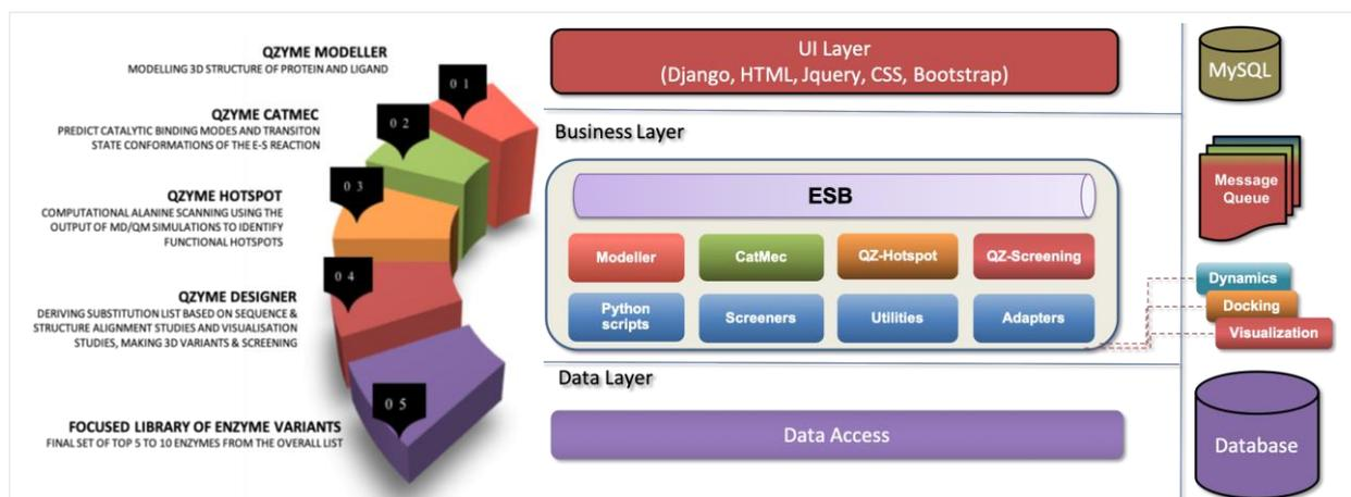
Figure 1: QZyme Workbench Modules (left) and Automation architecture overview(right)
